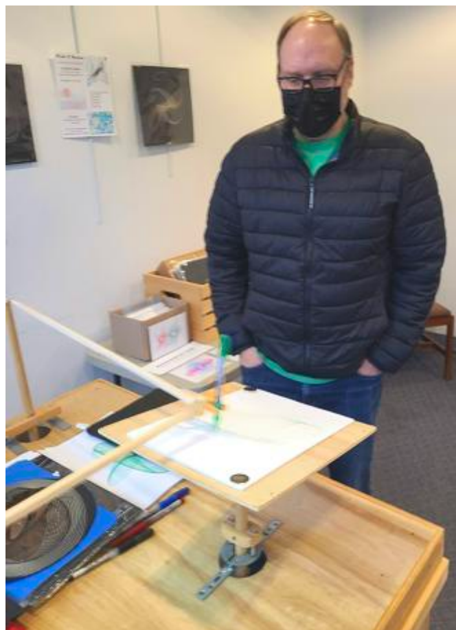
Don Fitzpatrick, of Grantham, creates harmonographs and pendulum drawings using pens to design the pattern, then initiating the harmonic motion of this device.
