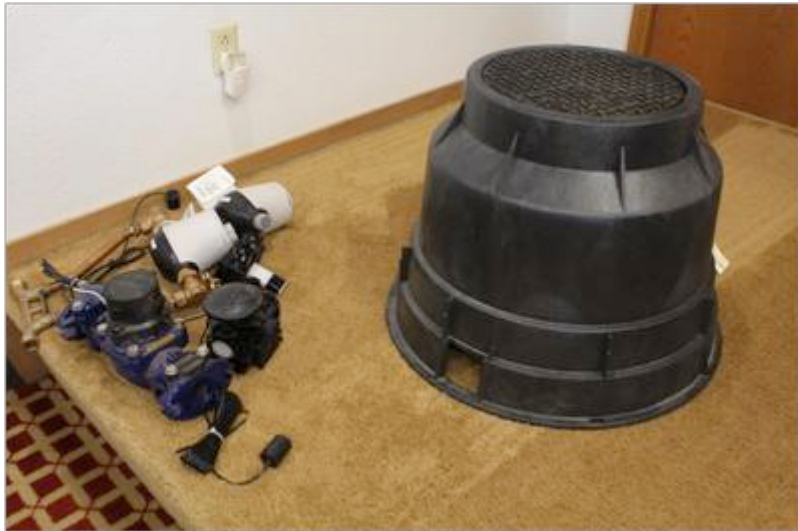
Photo: AMR water meter unit and internal mechanisms
