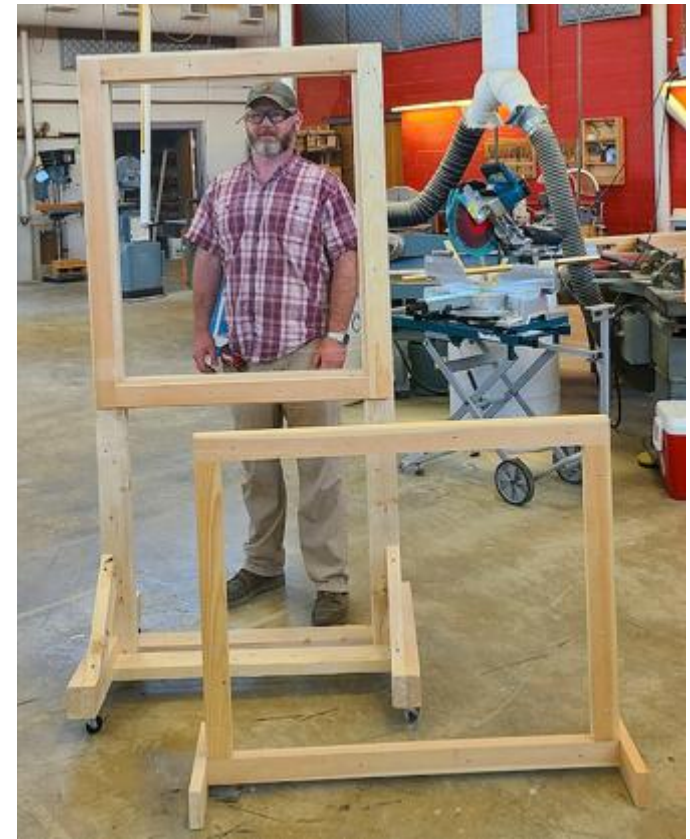
Mike Bennett is seen clearly behind the plexiglass of two safety shields, which he designed. The large model has wheels so a teacher can move it around the classroom. The smaller one is designed for table-top use in elementary schools; space at the bottom serves as a pass-through for papers. The shields will be delivered with no more than a basic stain, to encourage a friendly design competition among teachers (Eric Zengota photo).
