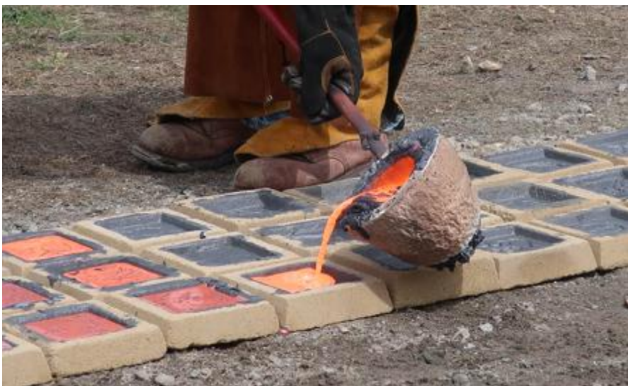
Looking like a solid rather than a liquid, a narrow stream of molten iron flows into a hand pouring ladle; artist Ernest Montenegro holds some of the broken iron bits to be melted down for the pour; filling the sand molds with the molten iron. The different colored squares show the differing stages of cooling (Top and middle photos by Dakota T. Bonner; bottom photo, Phyllis A. Muzeroll).
